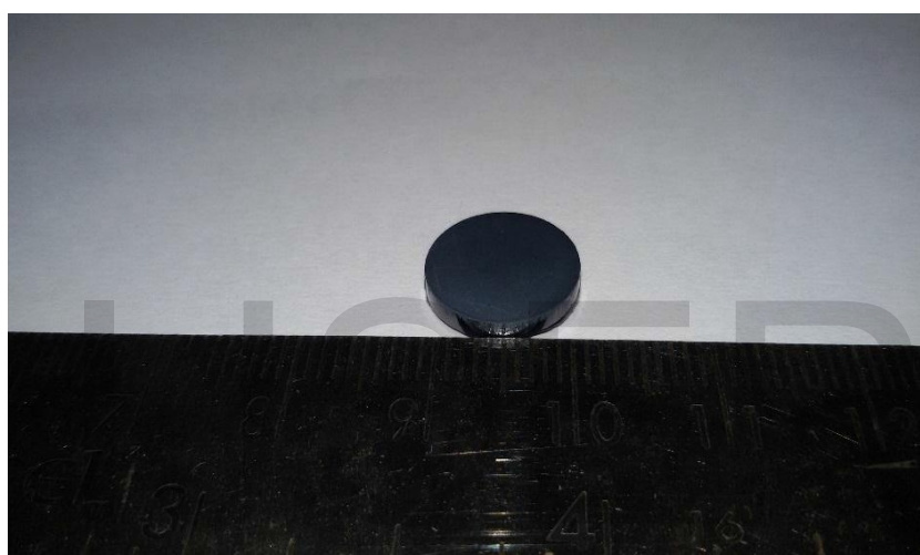
Fig. 1 CIP consolidated microwave sintered bulk disc from 75 hours ball milled powder
